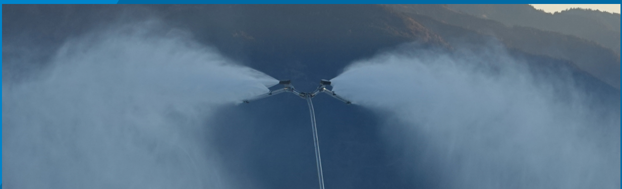
The SnoTek MEDUSA reaches the full capacity even at -8 °C WBT and is able to process up to 900 liters of water per minute and to produce up to 120 m 3 /h snow.
