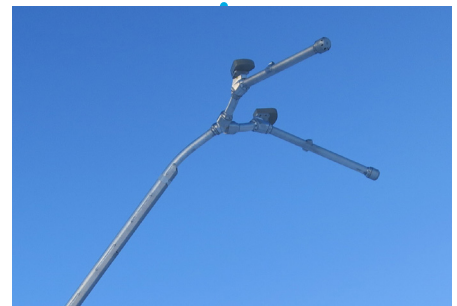
2015: SnoTek MEDUSA – The power package optimised for maximum performance. Up to 900 litres of water per minute can flow at -8^{\circ} WBT.
