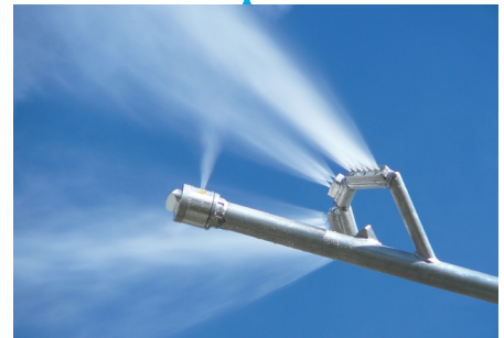
2014: NESSy Zero E – The world's first snow gun to operate entirely without electricity and additional energy.
