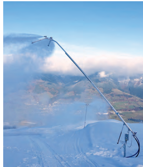
In the past, it was the fan gun machines that were complemented by the snow lances; today, it is often the other way around.
