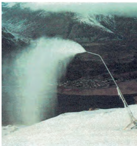
The HKD snow lance in the mid-80s used around 2,900 litres compressed air per minute.
