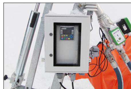
Fully automatic system mounted on the MAV
