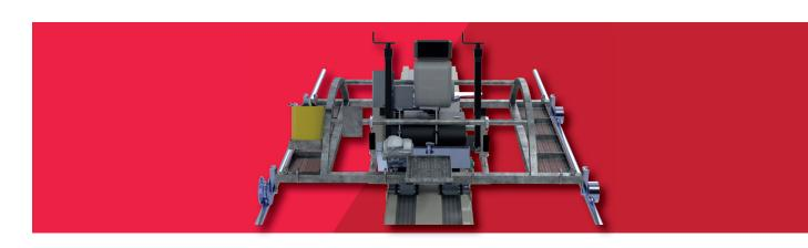
The preparation-system "Basic" is drawed up by a winch like the "Comfort" model but without a permission for passenger transportation. The preparation-system consists of a tiller and a brush unit and is guided by the plastic track limitation on the side.
